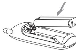
*When re-inserting the battery, it can only be inserted one way with the black plastic 'foot' of the battery pointed to the left hand side.*
